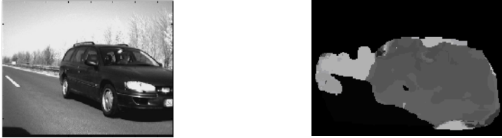
Fig. 1. Car segmentation using optical flow. Dark greys represent rightward movements (the car) and light greys leftward motion (the landscape). We can see that the proposed model gives us very uniform object segmentation therefore car tracking can be done easily.
